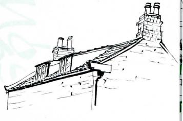
The vernacular style of guttering is half-round, cast iron with rise and fall brackets.
